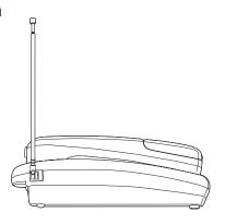
Hang the Handset on the cradle when the phone is mounted on a wall.
